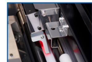
The CCD scanner can read barcodes to recall any job stored in memory as well as the registration mark to correct any image shifting.
