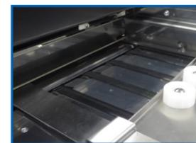
Adjustable in four steps, the vacuum registration table precisely aligns each sheet, maintaining a high degree of precision finishing.
