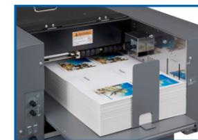
Automatic feed tray features a vacuum feeding system that prevents marking, miss or double feeding. The air knife aids in sheet separation.
